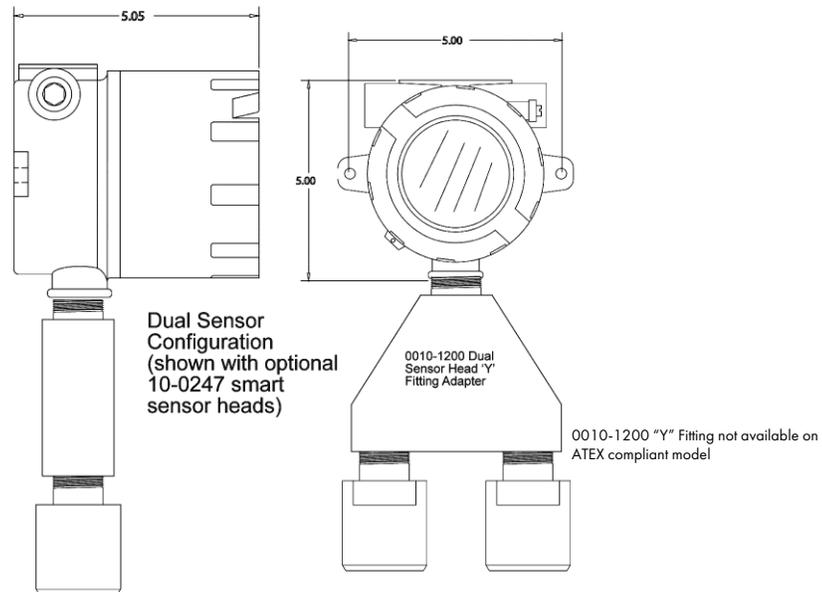
Figure 2-2a: SenSmart 3000 Explosion-Proof Housing with Dual Sensor Head Adaptor
