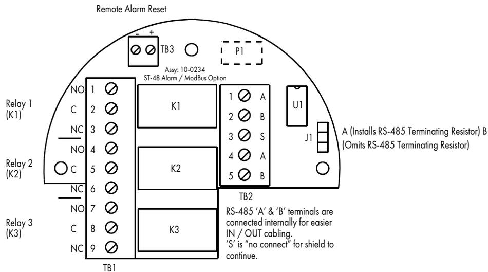
**Figure 2-6: 10-0234 Alarm Relays / Modbus Option**
