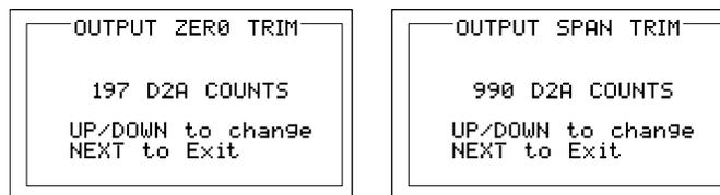
**Figure 3-2: Output ZERO / SPAN Trim Menus**
