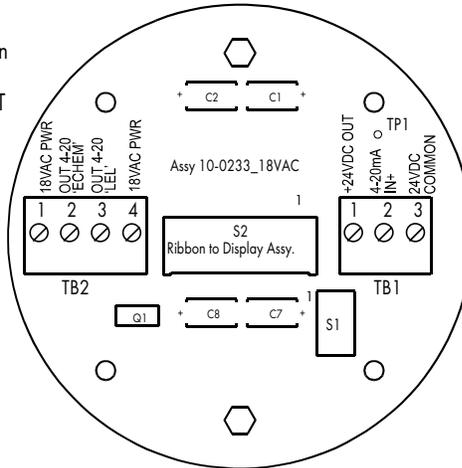
24VDC OUT is unregulated DC power generated from 18VAC~ input power.
