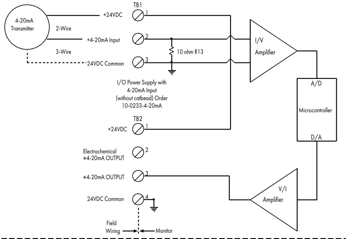
\* 10-0233-4-20mA is a special configuration allowing 4-20mA Input to TB1 and is available by special order.
