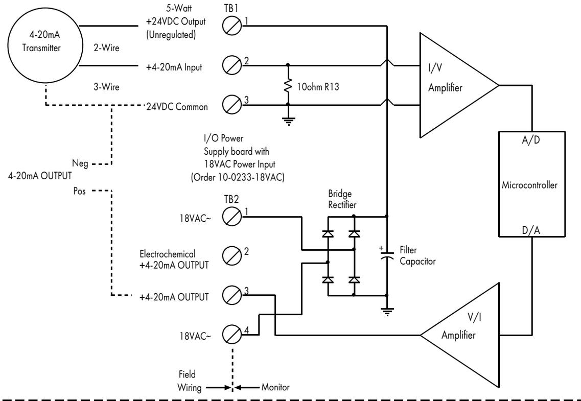
\*10-0233\_18VAC is a special configuration allowing power from an 18VAC~ power source and is available by special order. DO NOT APPLY 18VAC~ TO STANDARD UNITS!
