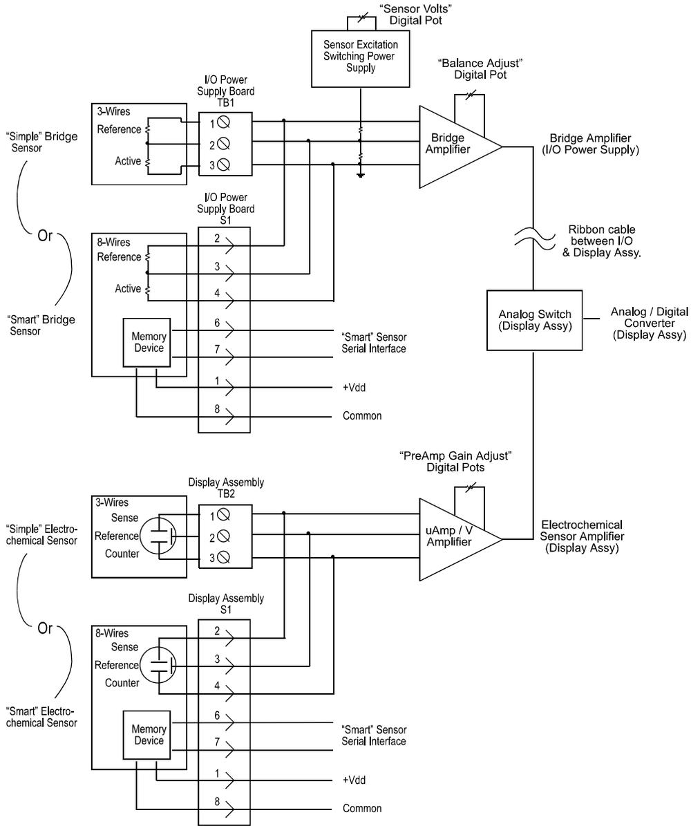
Figure 2-11: SenSmart 3000 Block / Wiring Diagram
