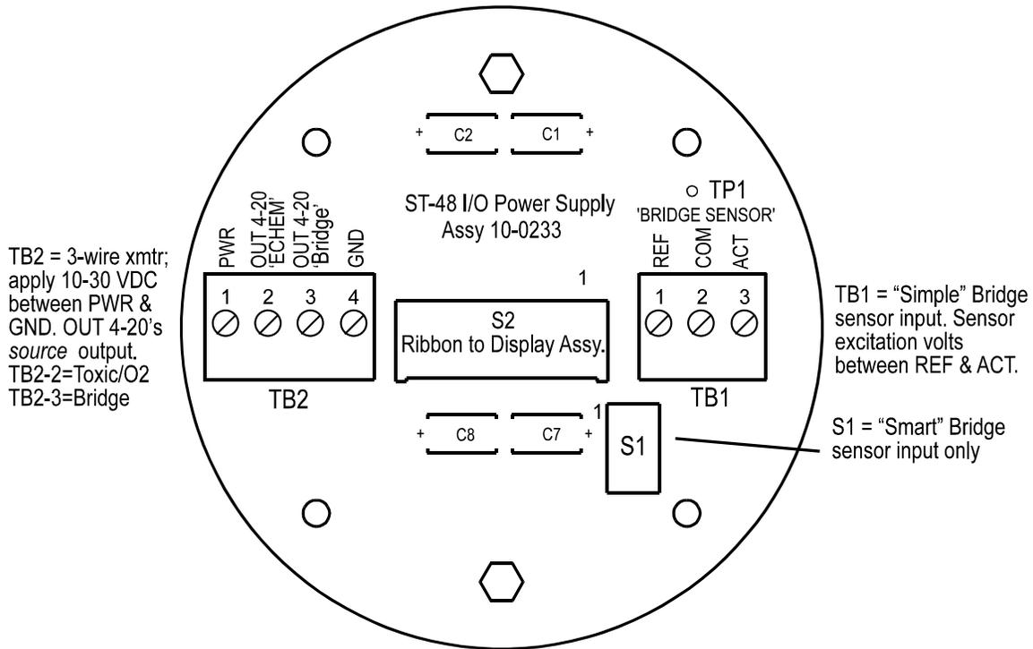
Figure 2-5: 10-0233 I/O Power Supply / 3-Wire 4-20mA Assembly
