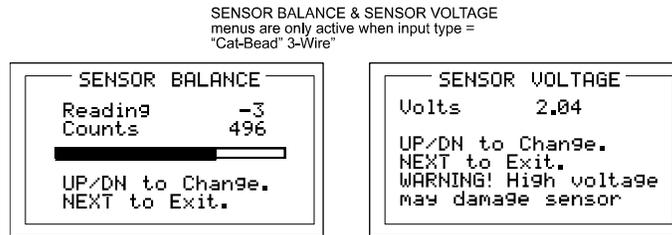
Figure 6-3: Catalytic Bead BALANCE & SENSOR VOLTS Adjust Menus
