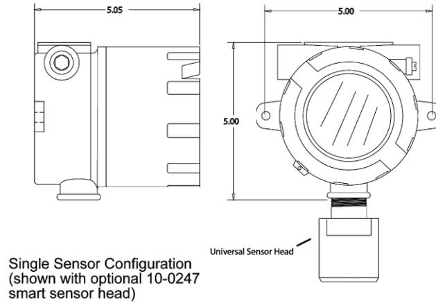
Figure 2-2: SenSmart 3000 Explosion-Proof Housing
