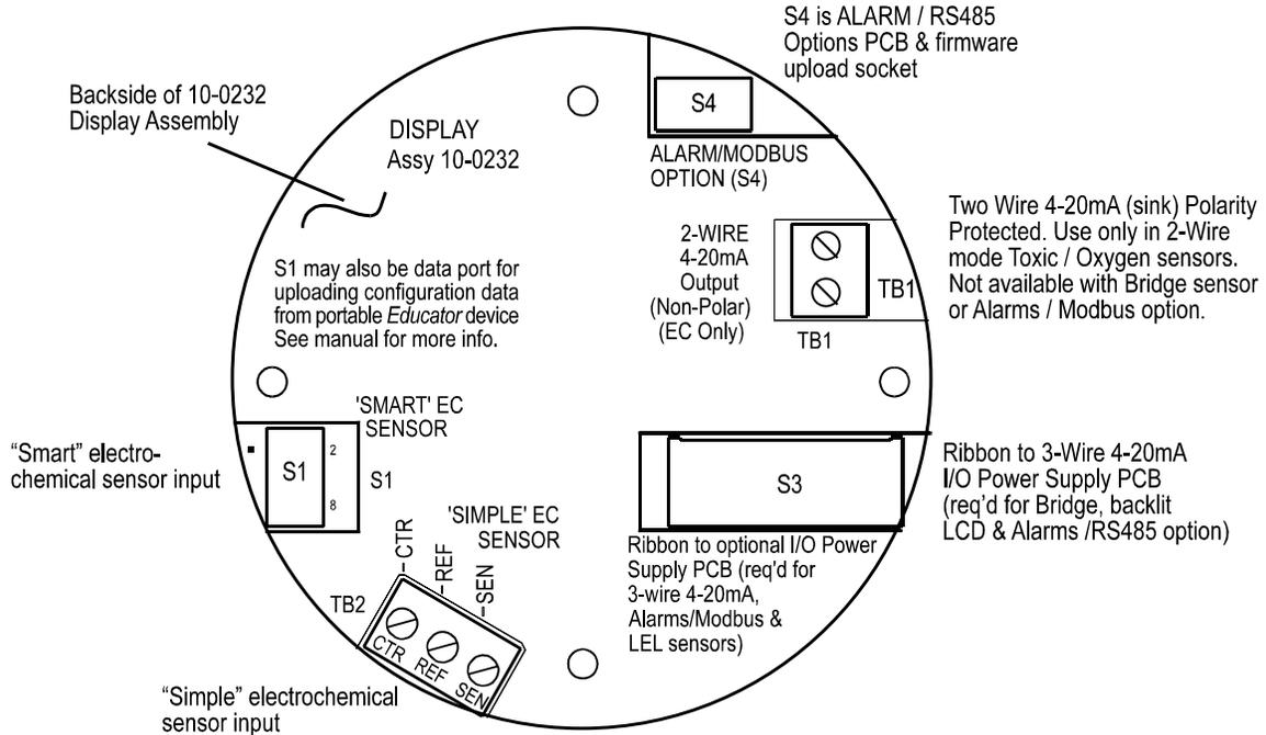
Figure 2-4: 10-0232 Display / SenSmart 2000 2-Wire 4-20mA Assembly
