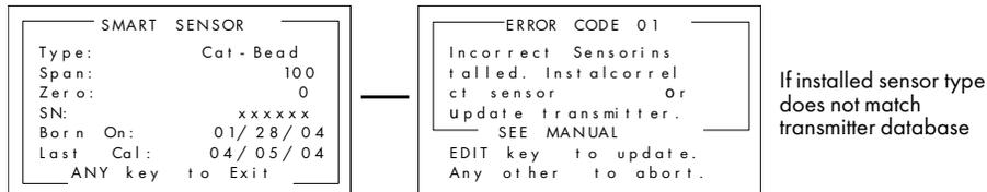
**Figure 2-10: Smart Sensor Info / ERROR Screens**
