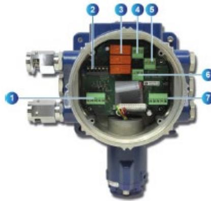
Figure 5: internal components of the transmitter.
