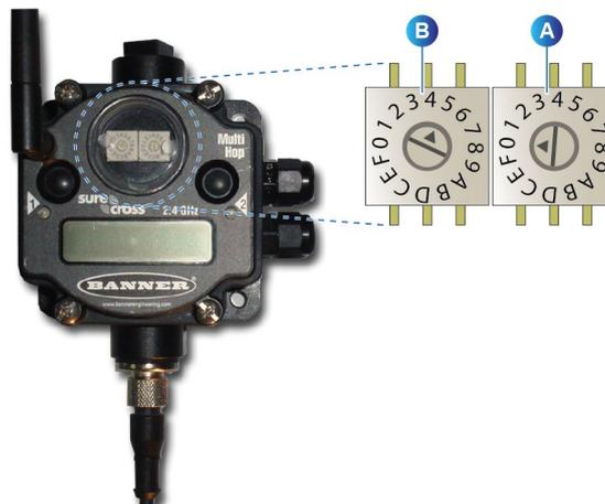
Figure 51: configuring the *master* receiver's address to @50.
