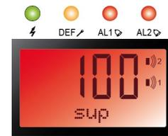
Figure 56: detection of high LEL concentration.
