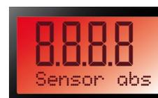
Figure 10: in the event of an alarm or fault, the type of fault is displayed. The orange DEF fault indicator light remains on as a solid light.
