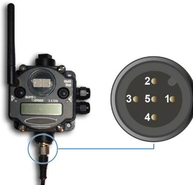
Figure 46: connecting the *master* receiver's 5-pin connector.
