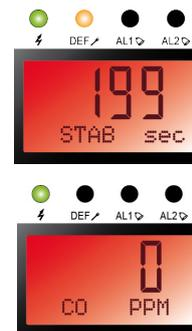
Figure 8: display sequence at start-up.
