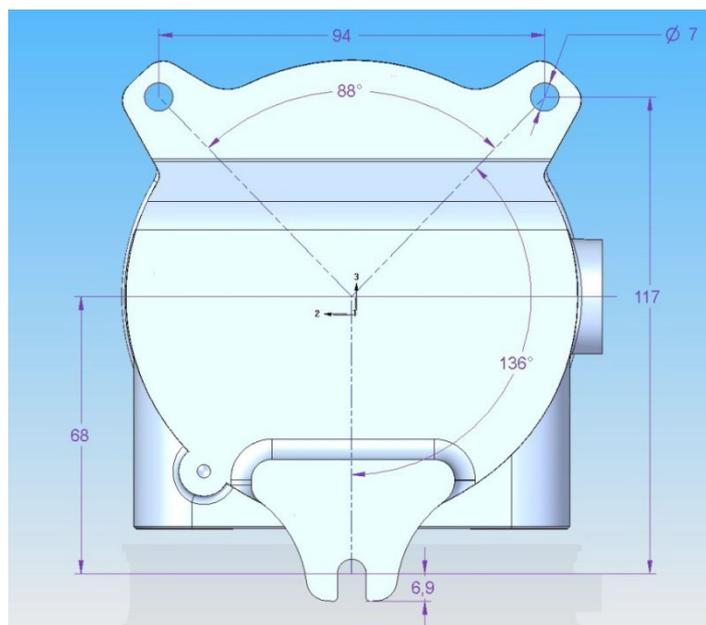
Drilling dimensions for support fixing.
