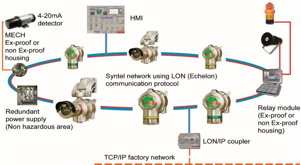
In this network version, an electronic board is inserted in the detector body and is used for electric connection.
