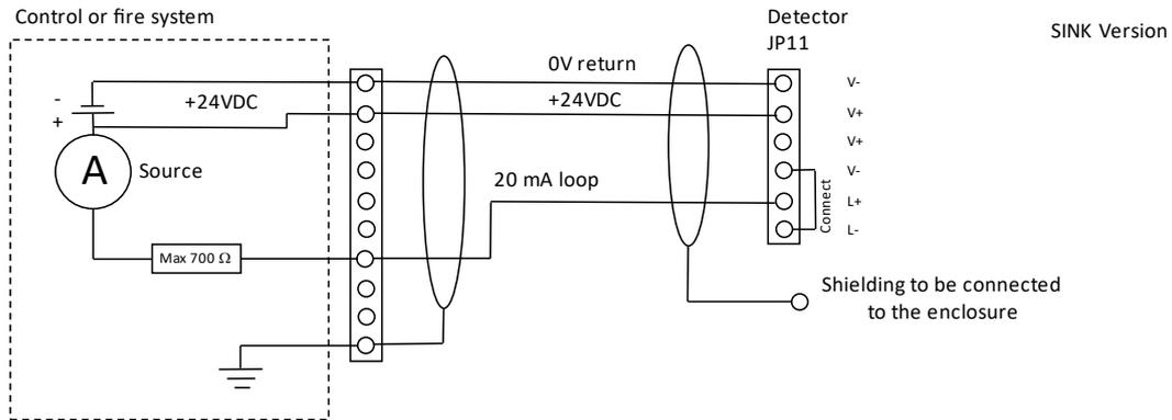
In this case, the output current is not isolated from power supply, consumed by the detector.
