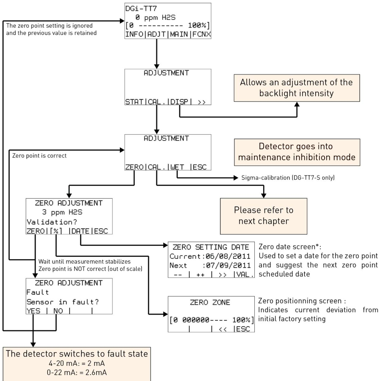
\* The device doesn't embed battery, it is then not able to keep real time. The date indication for zero or calibration points, as well as the next expected date for similar operations, are entered manually by the operator. Those data are for information only and their update is optional. mise à jour est facultative.
