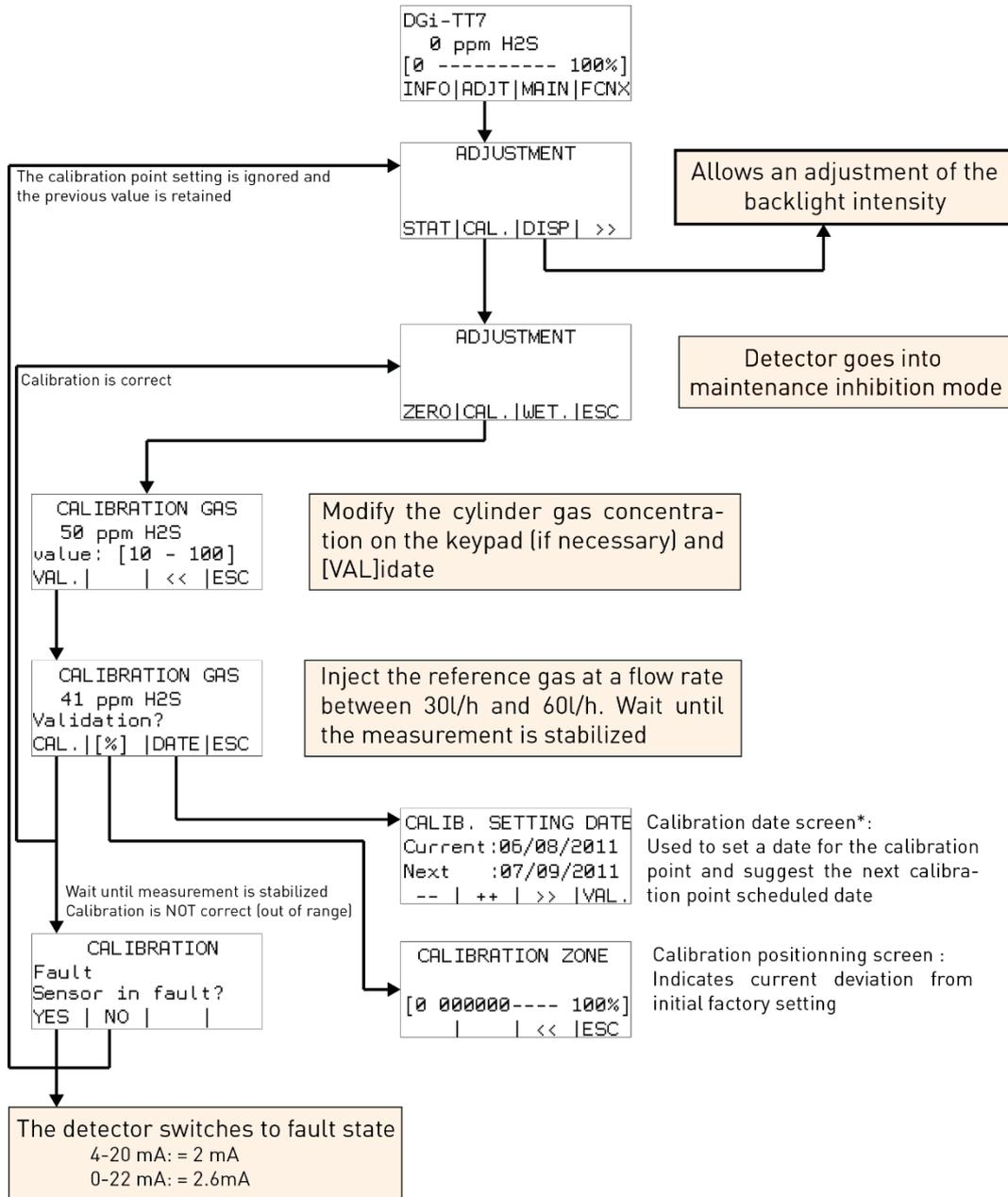
\* The device doesn't embed battery, it is then not able to keep real time. The date indication for zero or calibration points, as well as the next expected date for similar operations, are entered manually by the operator. Those data are for information only and their update is optional. mise à jour est facultative.
