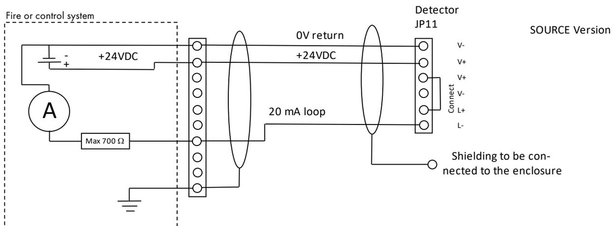
In this case, the output current is not isolated from power supply, provided from detector (standard connection).
