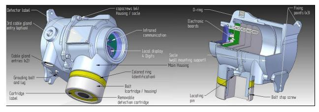
Figure 1 : Layout Drawing (Outline drawing – see Figure 2)
