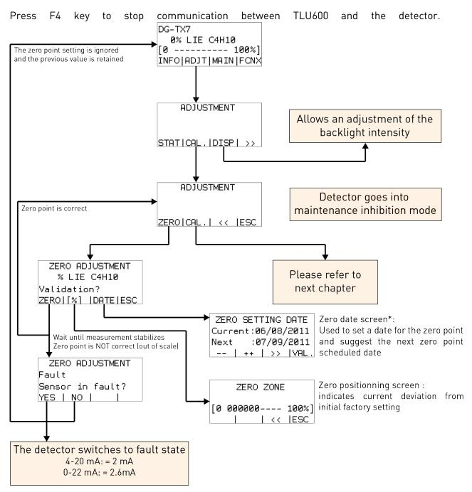
\* The device doesn't embed battery, it is then not able to keep real time. The date indication for zero or calibration points, as well as the next expected date for similar operations, are entered manually by the operator. Those data are for information only and their update is optional.mise à jour est facultative.
