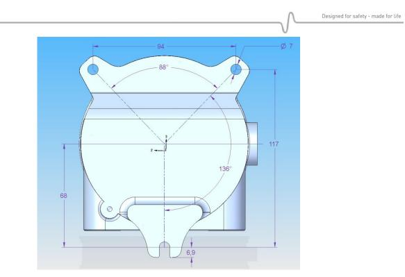
Figure 3: Drilling dimensions for support fixing.
