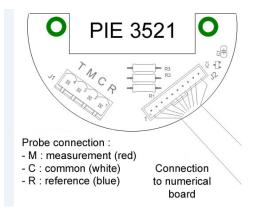
In order to operate this analog input, an additional electronic card (PIE3521) is added above the numeric card.
