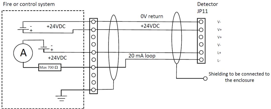
When using a 4 wires connection, the current loop is provided by the input module or PLC. The loop (L + and L-) is optically isolated from the detector. 4-20mA or 0-22mA input module of the PLC has to power up the current loop with, at least 8V at the terminal level.
