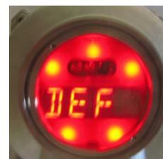
The device then goes in warming-up mode (refer to §6.3) for 90s. The detector is in inhibition mode. The current output and the default relay (if factory setting) are consequently activated.
