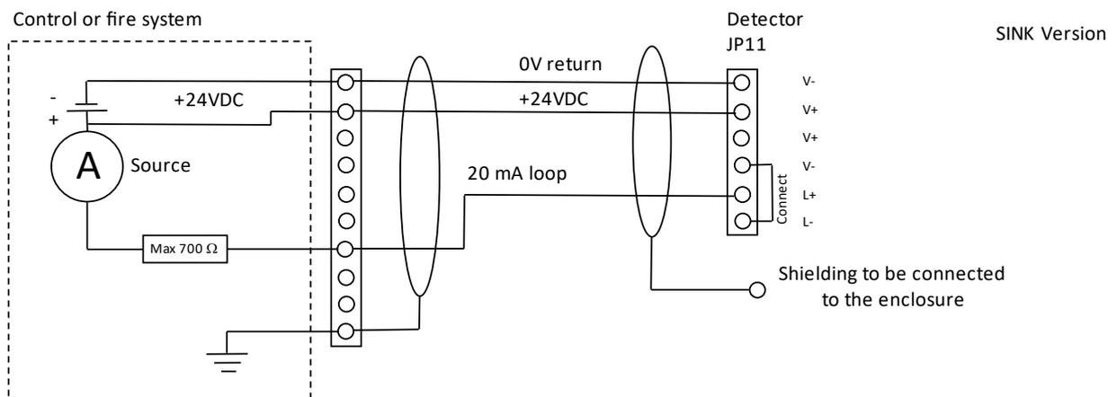
In this case, the output current is not isolated from power supply, consumed by the detector.
