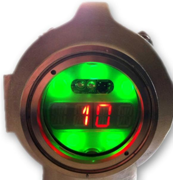
The orientation enables a communication with  $\frac{1}{2}$  horizontal angle about  $35^\circ$ ,  $\frac{1}{2}$  vertical-up angle about  $30^\circ$  and a vertical-down angle about  $50^\circ$
