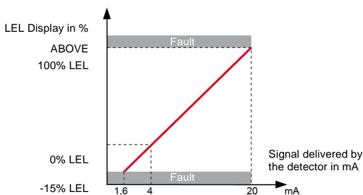
Figure 9: Configuration transfer curve 0 to 100 % LEL
