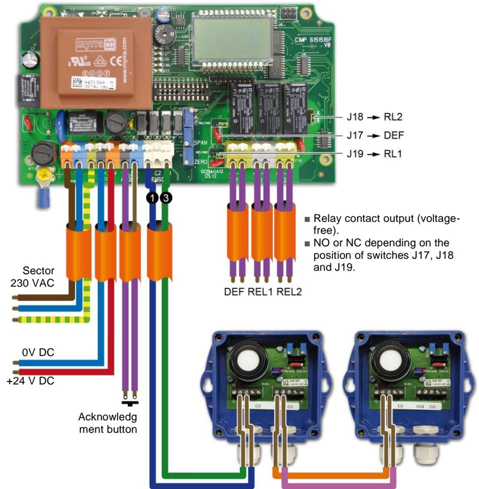
Figure 5: MX 15 controller and two OLCT 10 sensors for detection of the same toxic gas (maximum 5 sensors).
