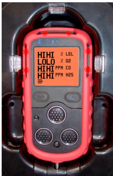
*Fig. 4-11 Instrument in Alarm Condition*
