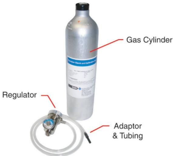
*Fig. 2-1 Calibration Gas Setup*
