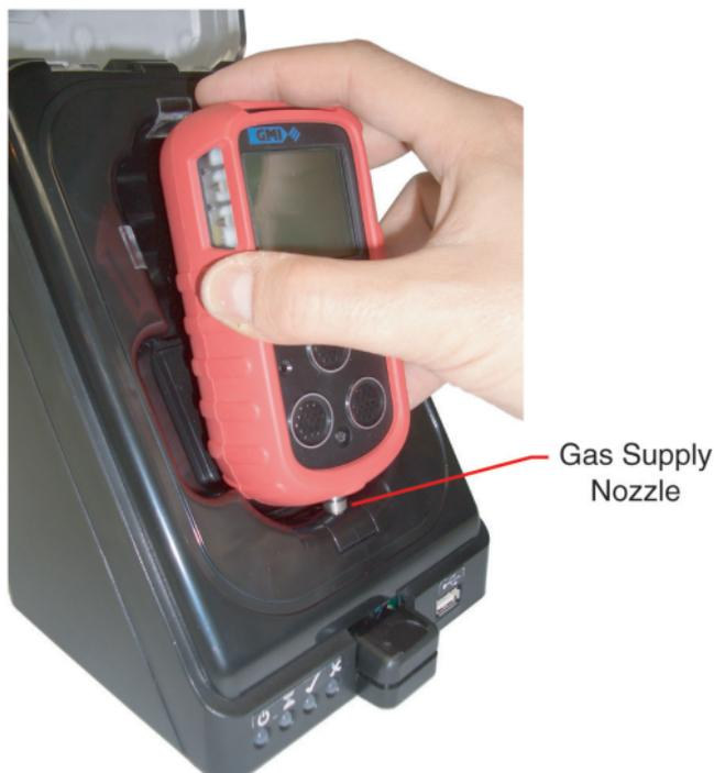
*Fig. 4-4 Locate Instrument on Gas Supply Nozzle*
