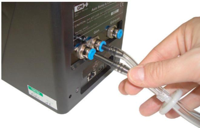
*Fig. 2-7 Connect Air Tubing Adaptor to Station*
