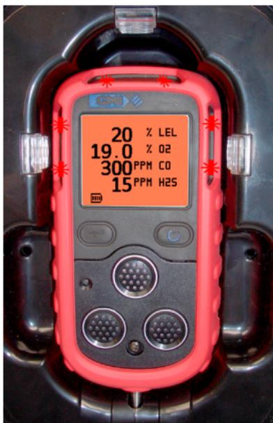
Fig. 4-10 Instrument in Alarm Condition
