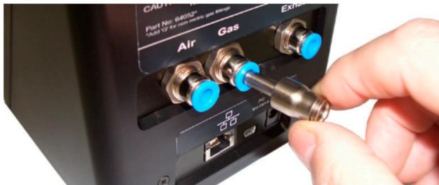
*Fig. 2-6 Fit 6mm to 1/4 in. Adaptors (if required)*
