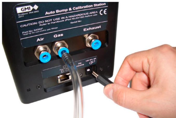
*Fig. 2-8 Connect Power Supply to Station*
