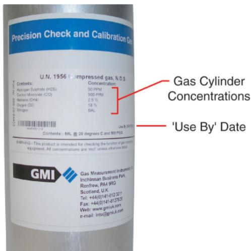
Fig. 2-2 Gas Cylinder Label
