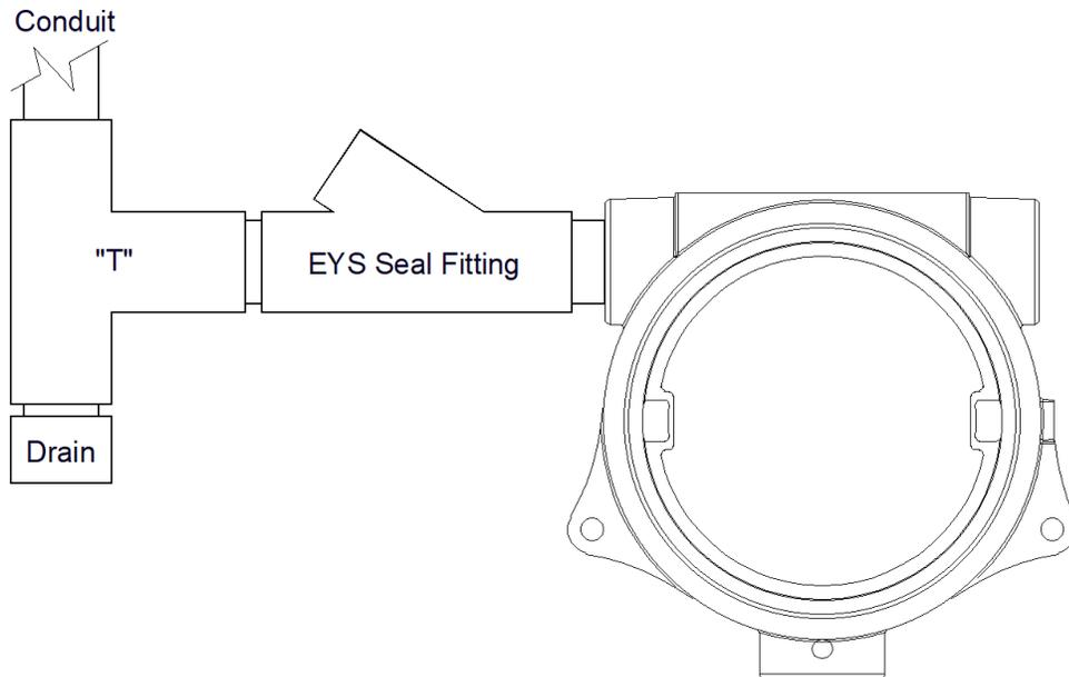
Figure 85 Typical Installation
