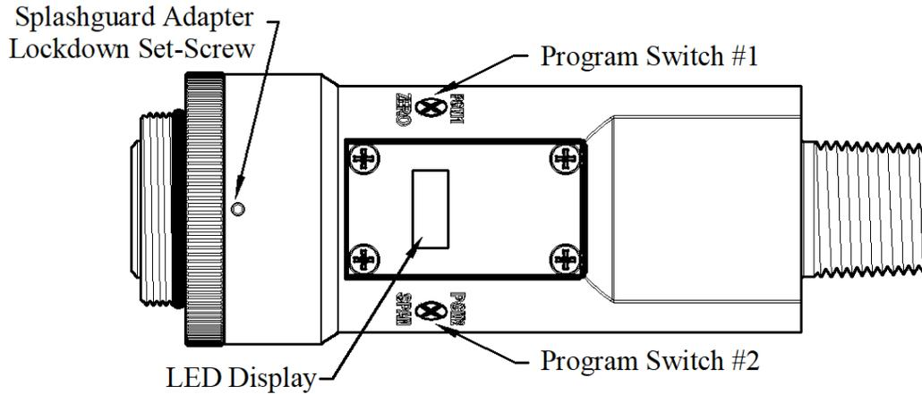
Figure 55 Sensor Assembly Front View
