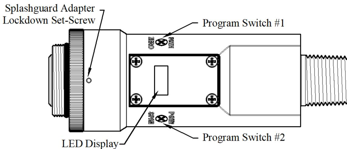
Figure 37 Magnetic Programming Switches
