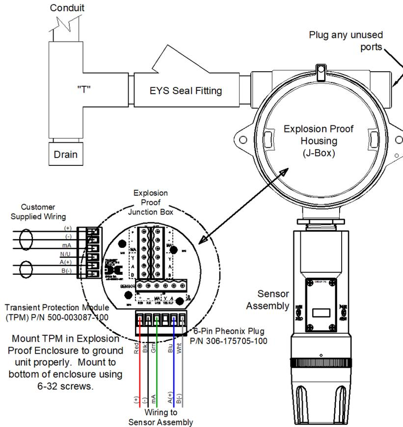
Figure 34 Typical Installation
