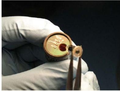
Figure 74 Lamp installation
