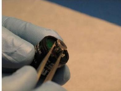
Figure 71 Removal of Lamp
