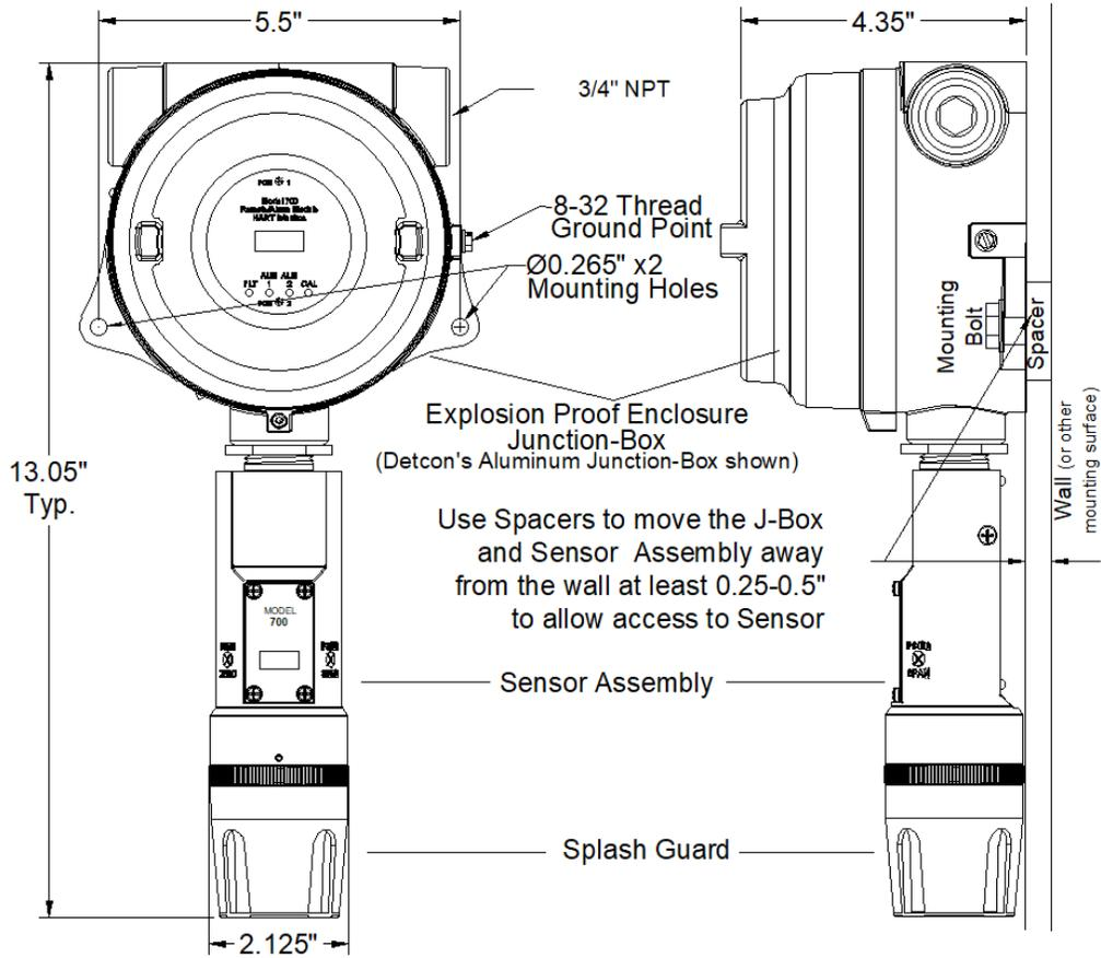
Figure 93 Mounting HART-RAM with 700 Sensor
