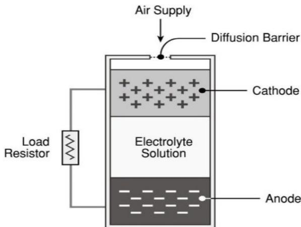
Figure 29 Construction of Galvanic Cell
