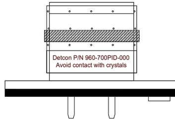
Figure 65 Plug-in sensor with Moisture control packet
