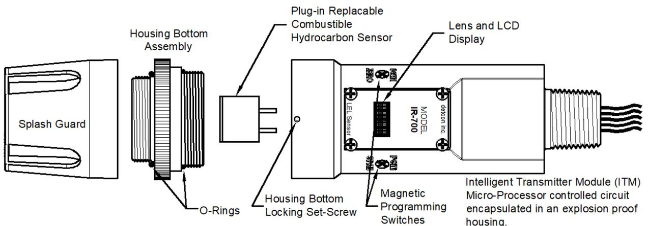
Figure 20 Sensor Assembly Breakaway
