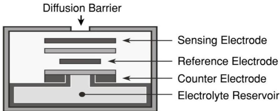
Figure 28 Construction of Electrochemical Toxic Sensor
