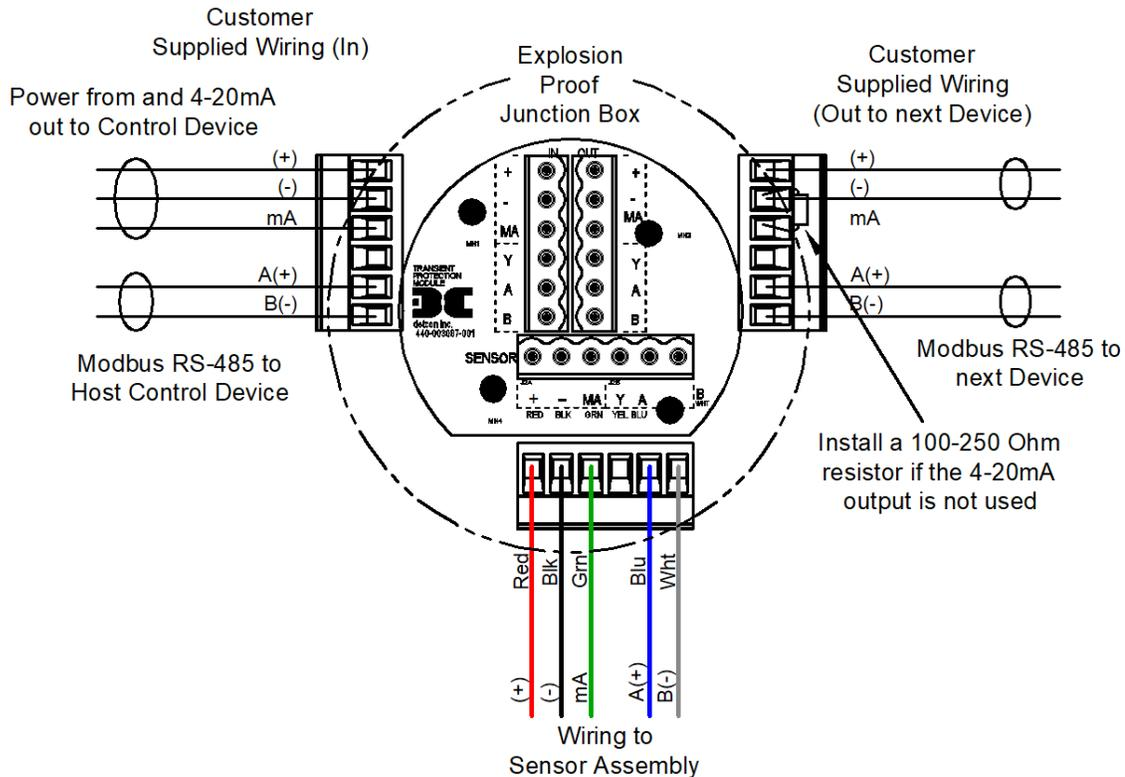
Figure 35 Sensor Wire Connections
