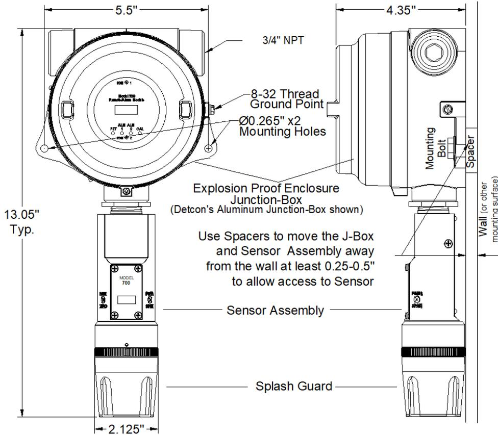
Figure 110 Mounting RAM with 700 Sensor
