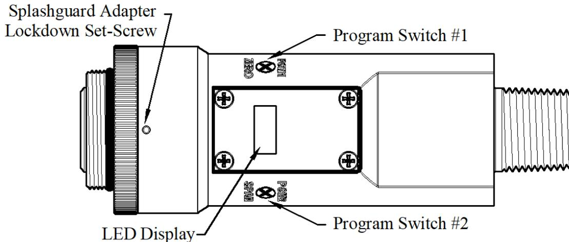
Figure 43 Sensor Assembly Front View
