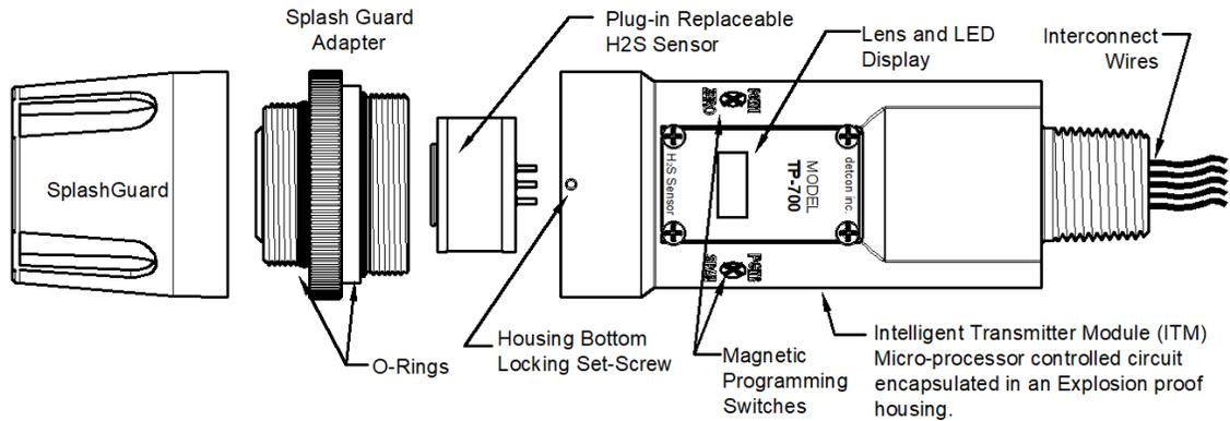
Figure 51 Sensor Assembly
