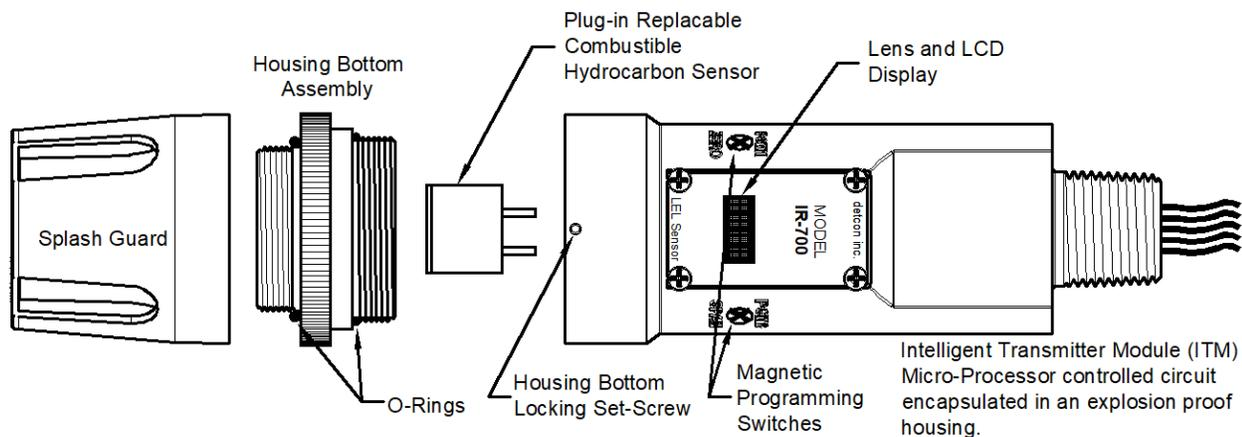
Figure 27 Sensor Assembly
