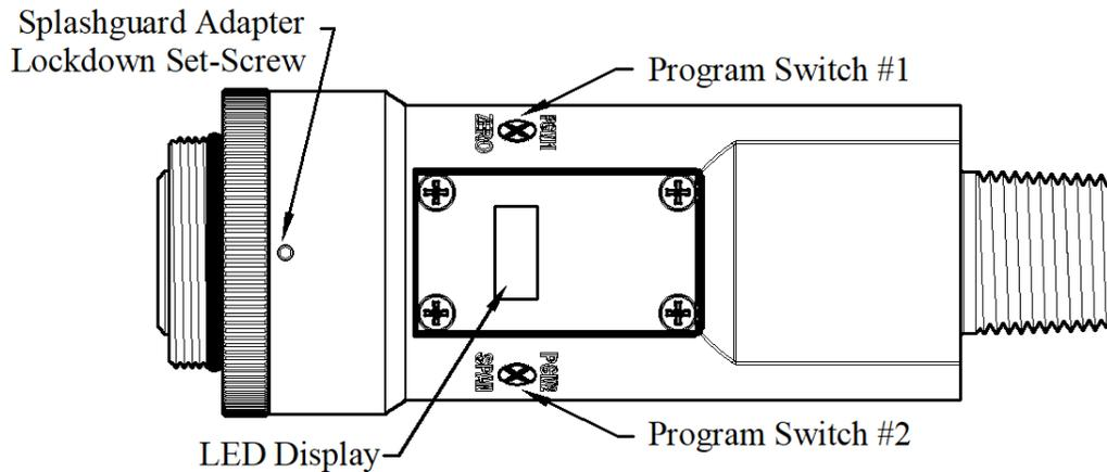
Figure 49 Magnetic Programming Switches
