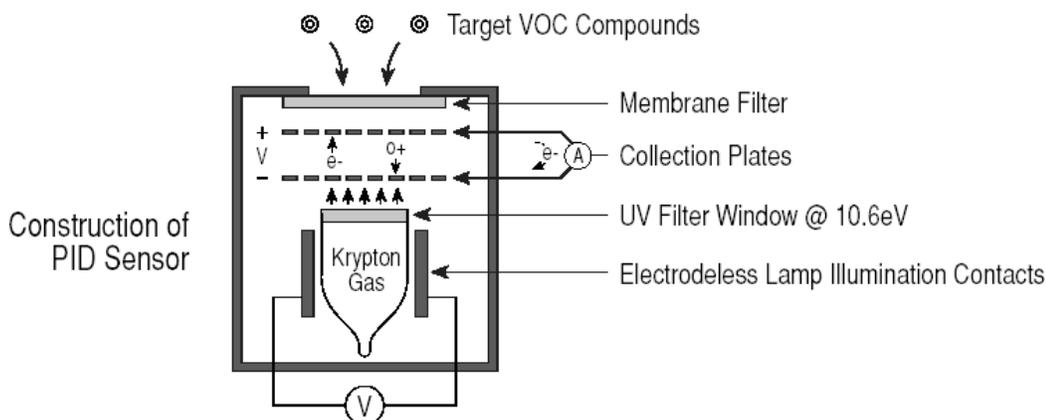
Figure 53 Typical Sensor Cell
