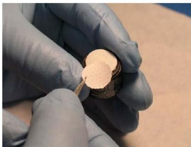
Figure 78 Installing Filter Media
