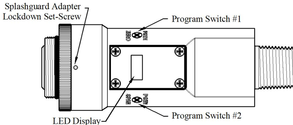
Figure 11 Magnetic Programming Switches
