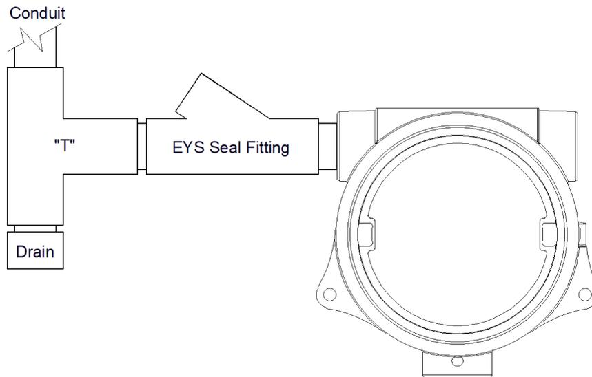
Figure 96 Typical Installation
