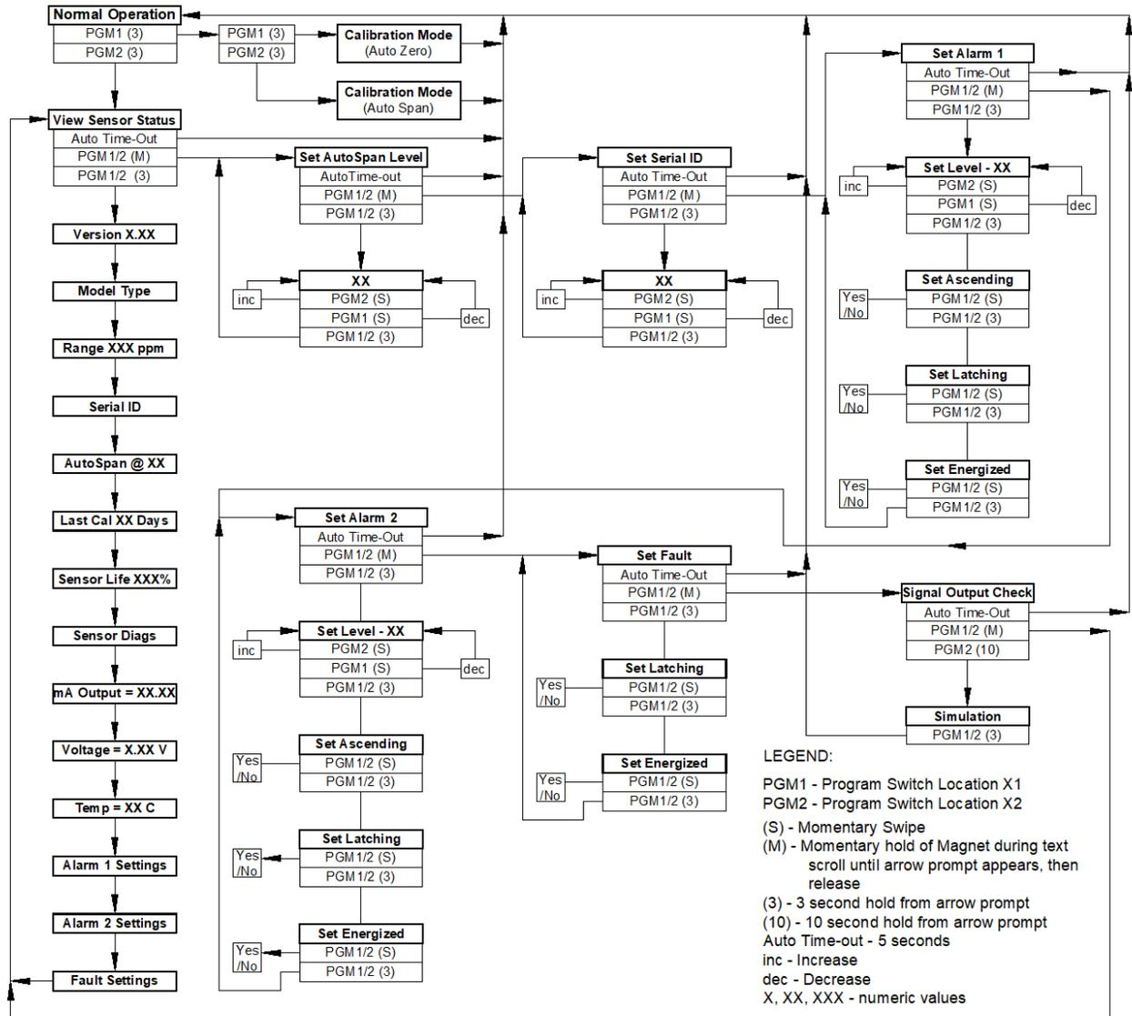
Figure 100 HART-RAM Software Flowchart
