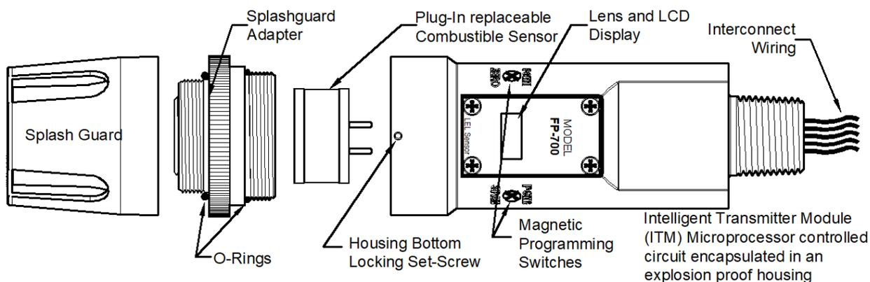
Figure 13 Sensor Assembly
