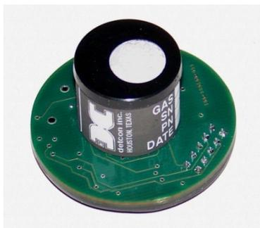
Figure 57 Intelligent Plug-in Sensor
