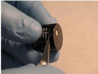
Figure 67 Removal of Filter Cap
