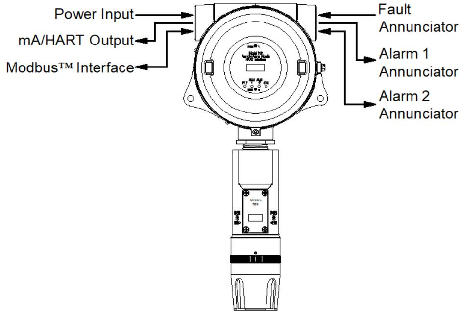
Figure 98 Installation with 700 Gas Sensor
