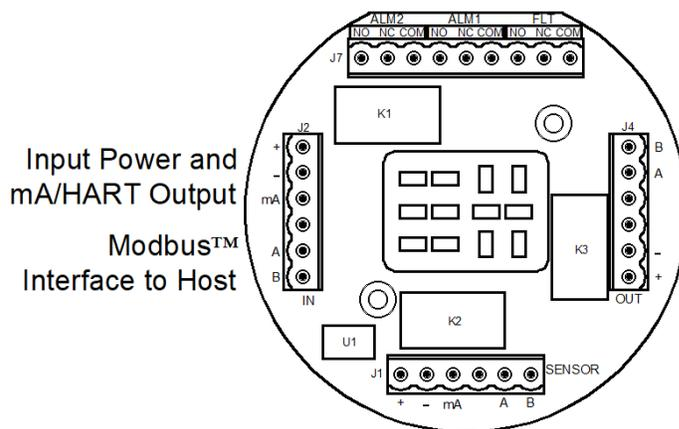
Figure 101 Hart Interface Connection
