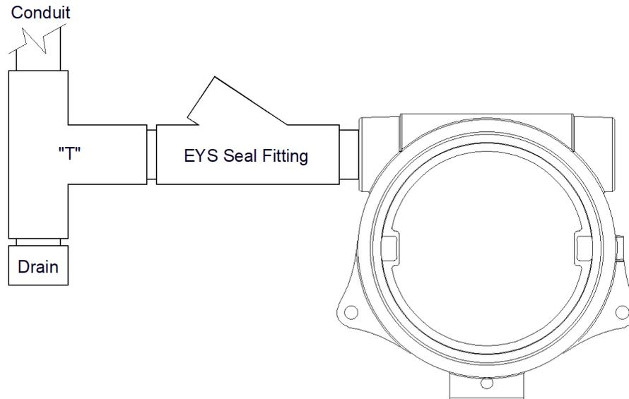
Figure 113 Typical Installation
