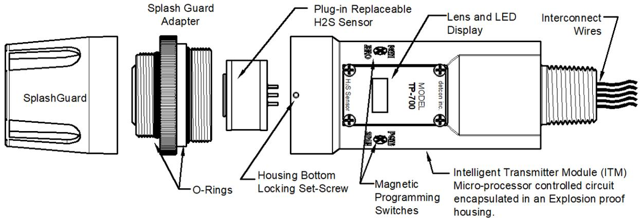
Figure 44 Sensor Assembly Breakaway
