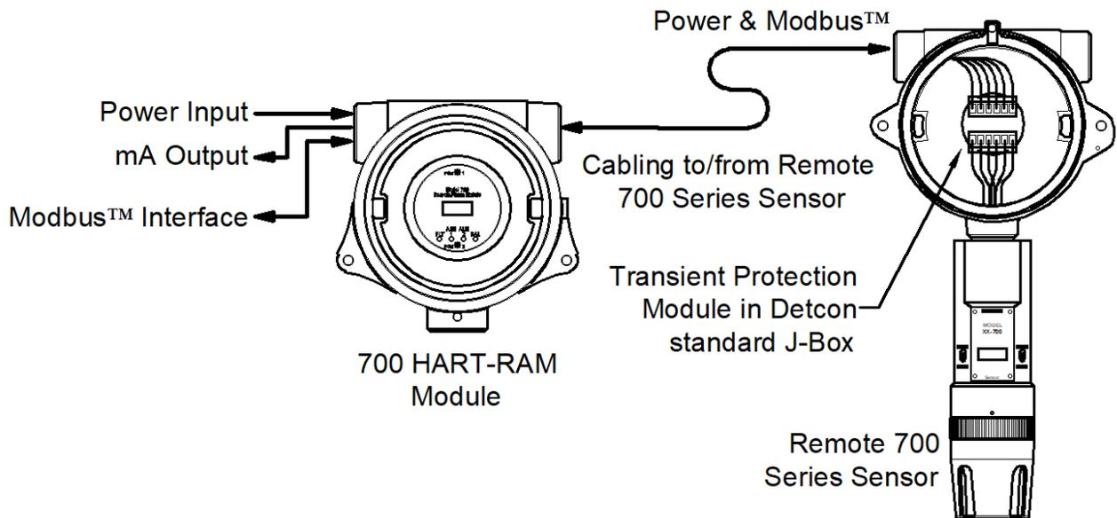
Figure 116 Remote 700 Gas Sensor with RAM
