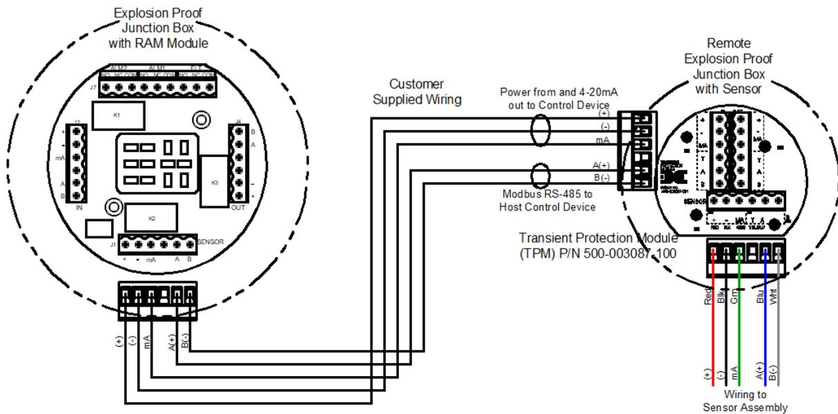
Figure 117 Remote Sensor Wiring
