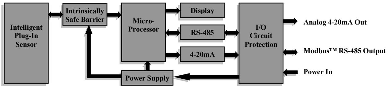
Figure 30 ITM Circuit Functional Block Diagram
