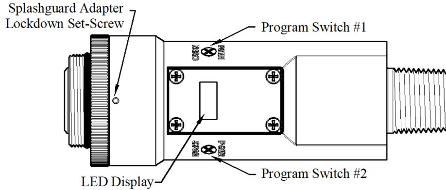
Figure 5 Sensor Assembly Front View
