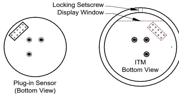
Figure 82 Sensor Cell and ITM Mating
