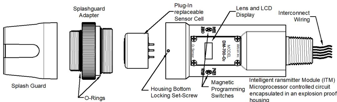
Figure 32 Sensor Assembly Breakaway
