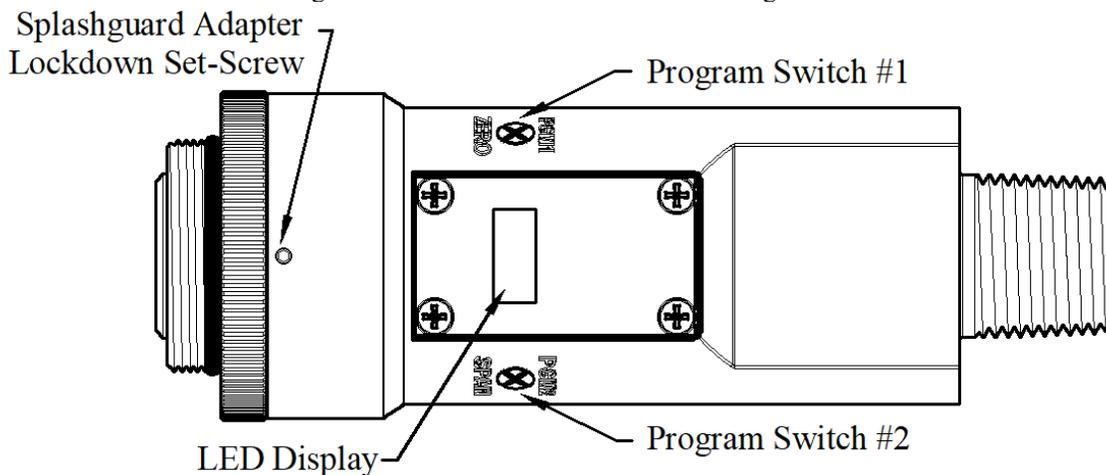
Figure 31 Sensor Assembly Front View
