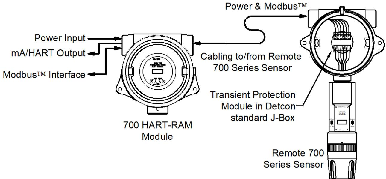
Figure 99 Remote 700 Gas Sensor with HART-RAM
