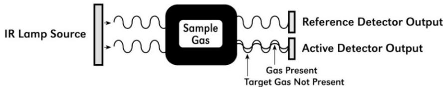
Figure 16 Principle of Operation
