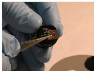
Figure 70 Removal of Cell Assembly
