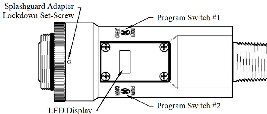
Figure 61 Magnetic Programming Switches
