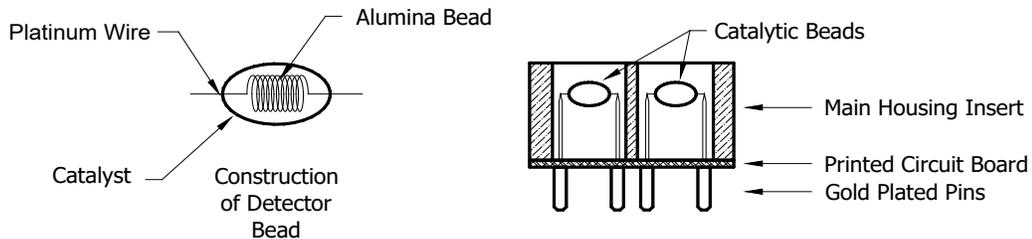
Figure 1 Sensor Cell Construction
