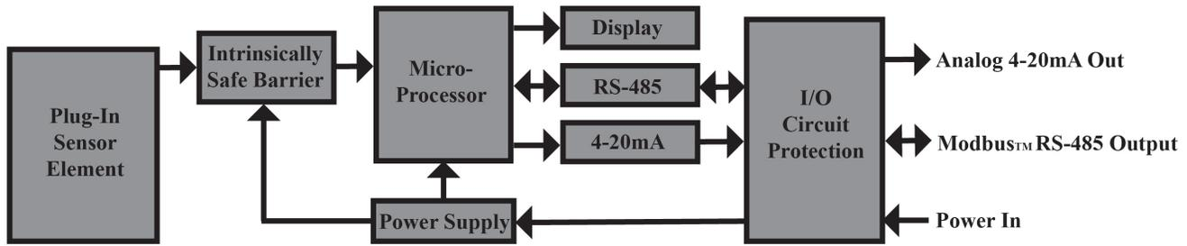
Figure 54 ITM Circuit Functional Block Diagram
