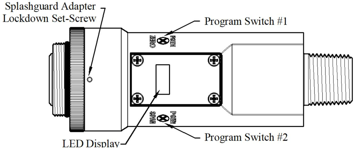
Figure 19 Sensor Assembly Front View
