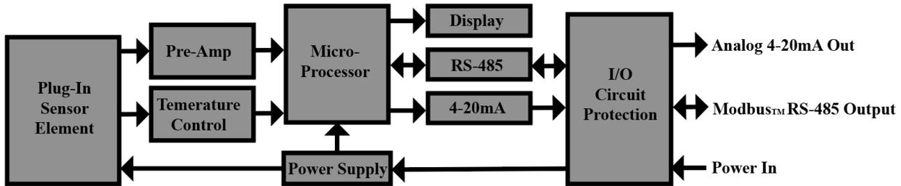
Figure 42 ITM Circuit Functional Block Diagram
