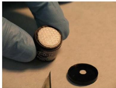
Figure 68 Removal of Filter Media
