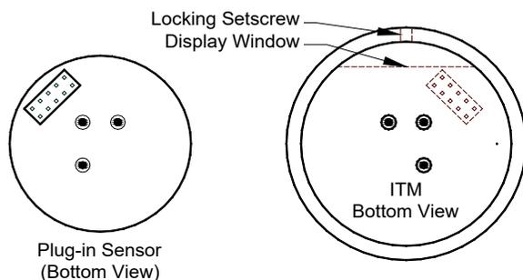
Figure 81 Sensor Cell and ITM Mating
