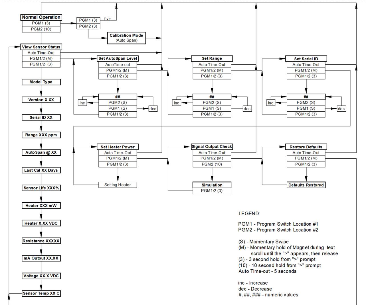
Figure 50 TP-700 Software Flowchart
