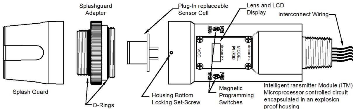
Figure 80 Sensor Assembly
