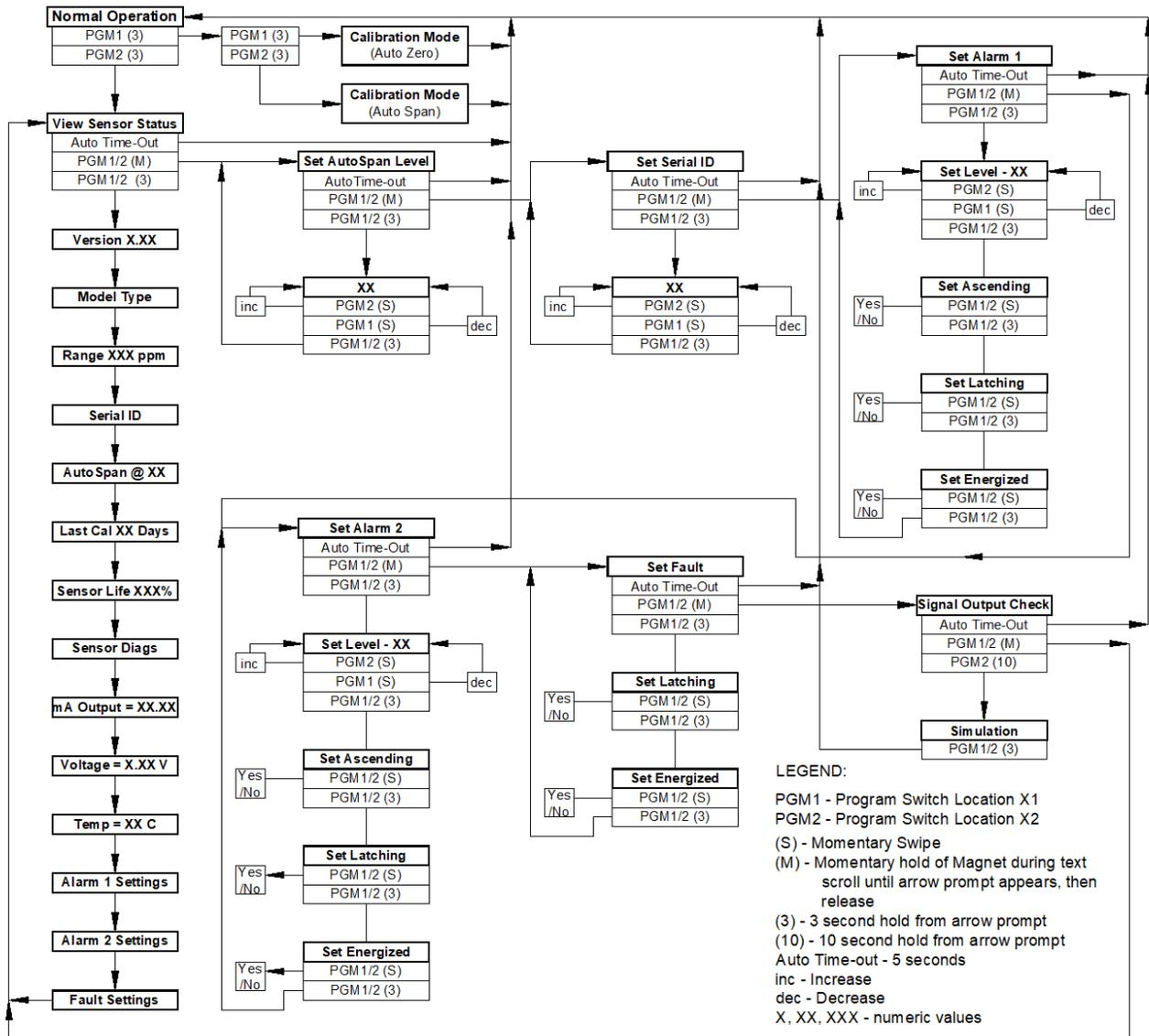
Figure 118 RAM Software Flowchart
