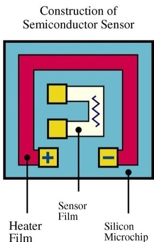
Figure 41 Sensor Cell Construction
