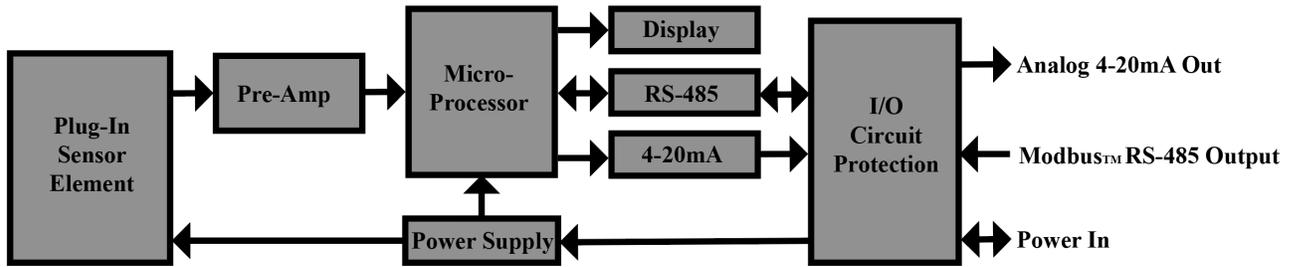
Figure 18 ITM Circuit Functional Block Diagram
