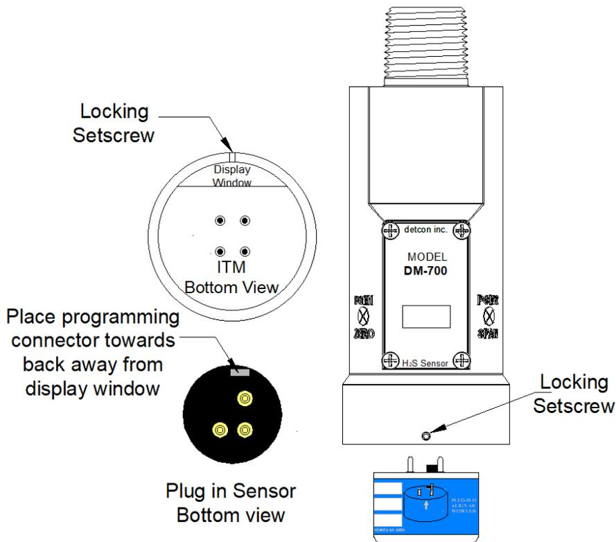
Figure 40 Sensor Cell and ITM Mating
