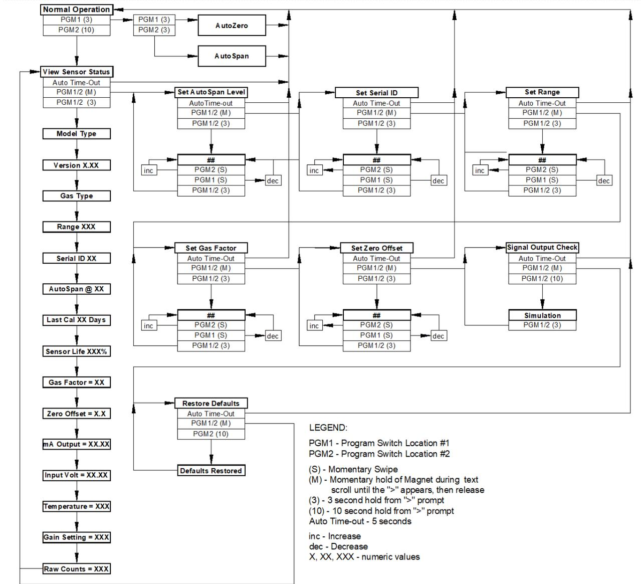
Figure 62 PI-700 Software Flowchart
