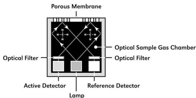
Figure 15 Sensor Cell Construction
