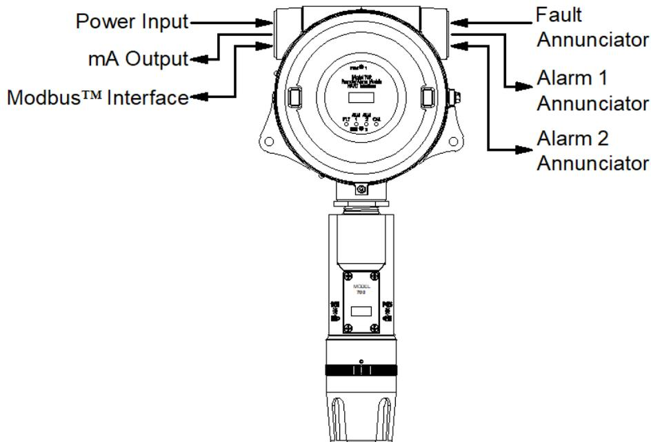
Figure 115 Installation with 700 Gas Sensor
