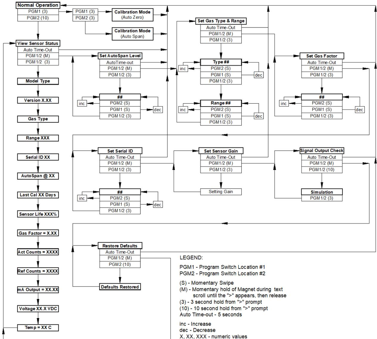
Figure 26 IR-700 Software Flowchart
