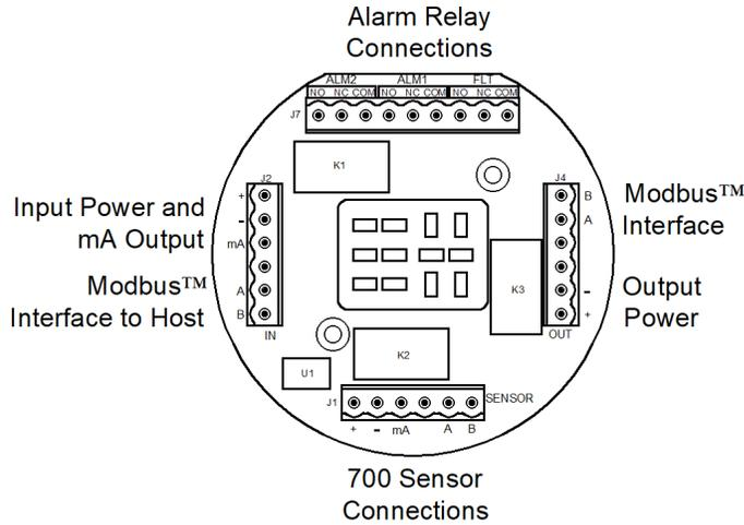
Figure 114 Interface connections on terminal board
