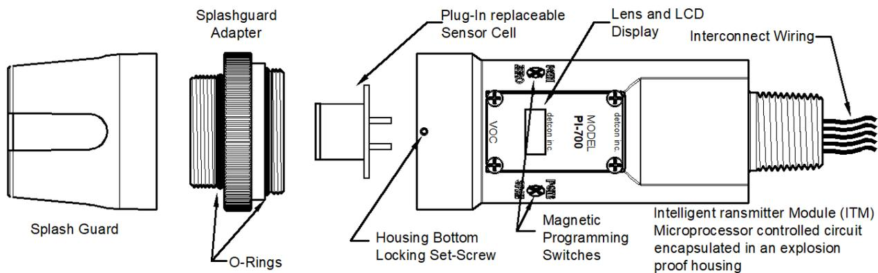
Figure 56 Sensor Assembly Breakaway
