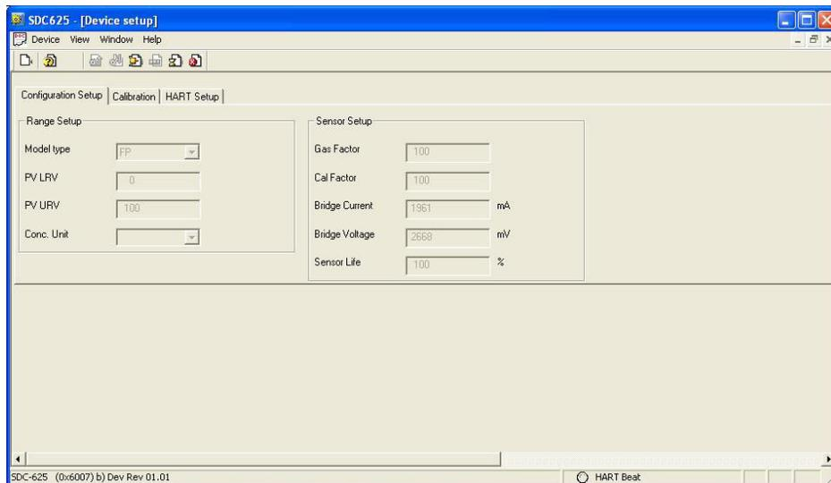
Figure 105 FP Configuration Setup
