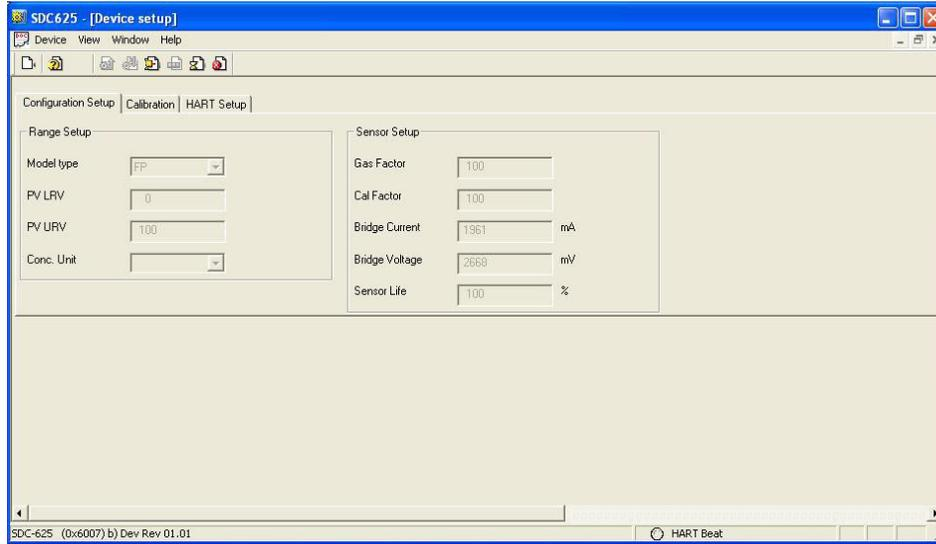
**Figure 7 FP Configuration Setup**
