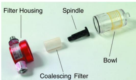
Fig. 5-12 Coalescing Filter Assembly
