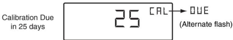
Figure 3-10 Days until Calibration Required
