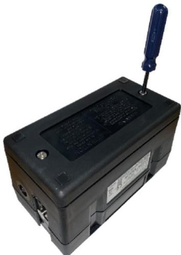
*Fig. 5-1 Loosen Instrument Base Screws*
