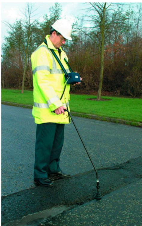
*Fig. C-4 Semiconductor Survey (Bellows) Probe*
