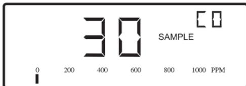
*Fig. 2-5 Carbon Monoxide Range*
