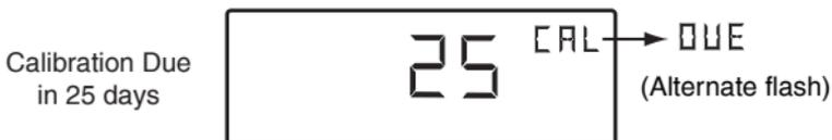
Figure 3-4 Days until Calibration Required
