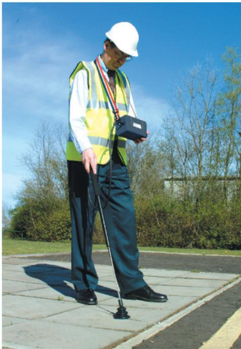
*Fig. C-6 Bellows Probe*
