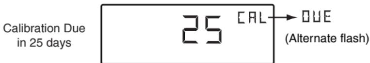
Figure 3-7 Days until Calibration Required
