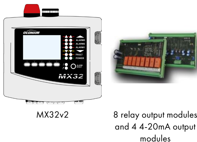
Figure 1: MX32v2 and examples of the modules
