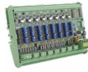
This module enables standard analog transmitters (gas or flame detectors for instance) to be connected on a digital line for cost savings.
