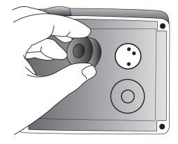
• Remove the shorting clip or small bias circuit board from the replacement sensor, aligning the holes in the board with the pins on the sensor; plug the new sensor into the instrument.
