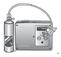
At this point all on-board and remote alarms should be activated and the 4-20 mA signal should reflect the display reading on the instruments.
