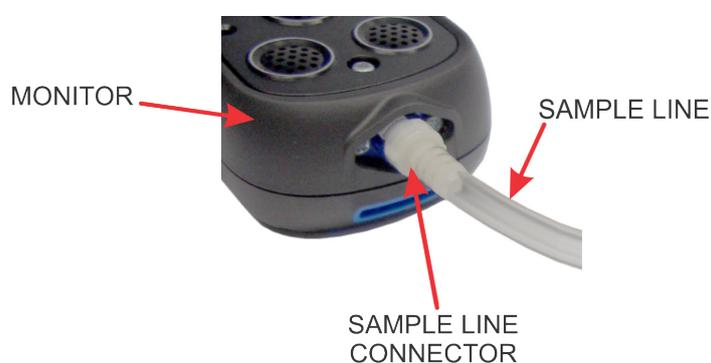
**Figure 19: Sample Line Connected to Monitor**
