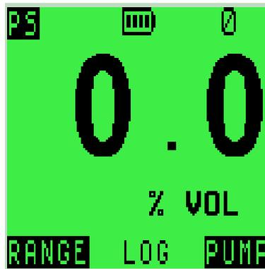
**Figure 29: Datalogging Indicator**
