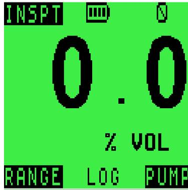
**Figure 26: Datalogging Indicator**
