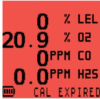
**Figure 5-11: CAL EXPIRED (CALIBRAGE EXPIRÉ)**
