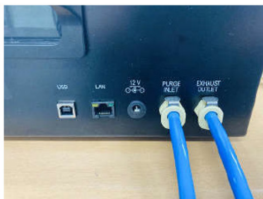
Figure 4-4: Connect Air & Exhaust tubing
