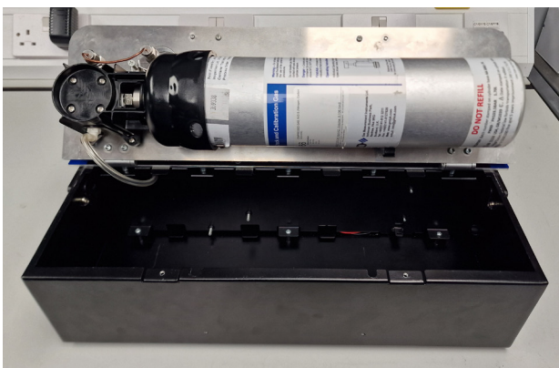
Figure 4-3: Secure the gas cylinder
