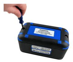
Figure 64: Battery Pack Removal
