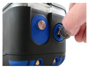
Figure 70: Inlet Nozzle Removal
