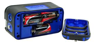
Figure 57: Battery Cover Removal
