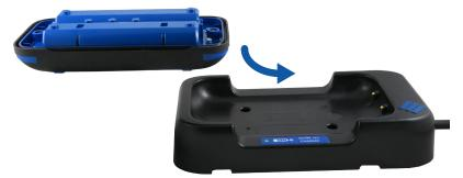
Figure 66: Battery Pack Charging
