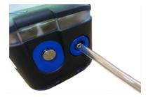
Figure 87: Connect Calibration Gas
