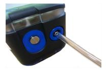
Figure 79: Connect Calibration Gas
