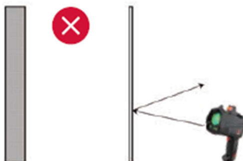
Case 2: Avoid detecting through anti-infrared or absorbing infrared material
