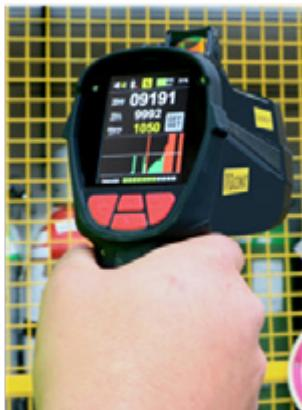
Using powerful laser spectroscopy technology, the **GAS LASER** is a handheld remote methane detector (RMD) offering methane selectivity. Ultra-portable and very easy to use, this device detects methane leaks on outside gas pipelines along buildings, bridges or within gas and industrial sites. Its ability to detect methane through glass also makes it an essential tool for conducting inspections, safely and efficiently.
