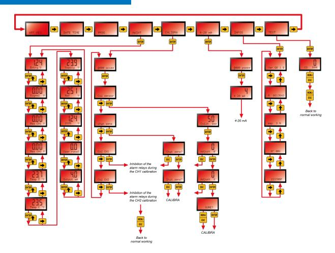
Figure 16: the OLCT 80's sub-menus under MAINT, CALIBRA, 4-20mA, INFOS and TEST.
