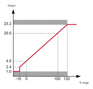
Figure 43: transfer curve for a 4-20 mA detector.
