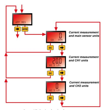
Figure 17: the Reading Display menu.
