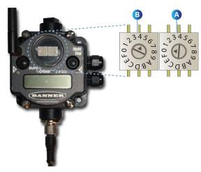
Figure 51: configuring the master receiver's address to @50.
