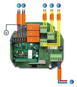
Figure 47: wireless OLCT 80 connections.
