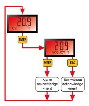
Figure 58: alarm acknowledgment diagram.
