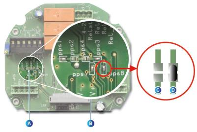
Figure 60: example of a solder pad with and without a solder joint.
