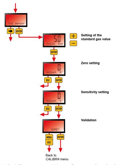
Figure 32: the Calibration menu. Press ESC repeatedly to return to the reading display.
