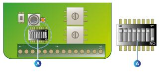
Figure 48: micro switch configuration on the OLCT 80.
