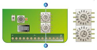
Figure 50: configuring the address of the wireless card.
