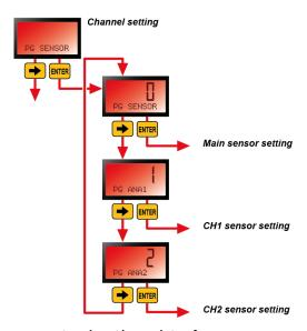
Figure 21: the *Channel Configuration* menu.
