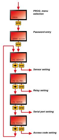
Figure 20: the *Configuration* menu leads to 4 different sub-menus. Press *ESC* repeatedly to return to the reading display.
