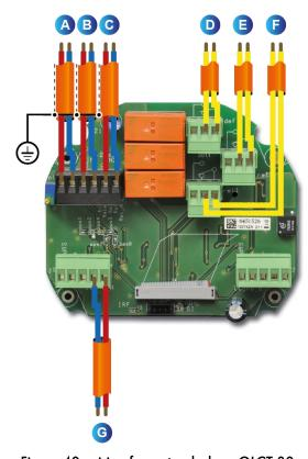
Figure 40: wiring for a stand-alone OLCT 80.
