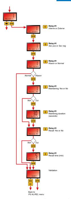
Figure 26: RELAY 1 menu. Press ESC repeatedly to return to the reading display.
