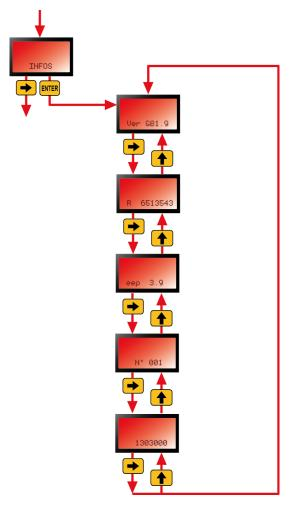
Figure 35: the  ${\it Info}$  menu. Press  ${\it ESC}$  repeatedly to return to the reading display.
