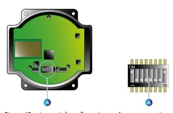
Figure 49: micro switch configuration on the *master* receiver.
