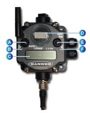
Figure 52: buttons and indicator lights on the master receiver.
