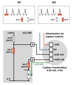
Figure 63: auxiliary input configuration for a 4-wire 4-20mA sensor.
