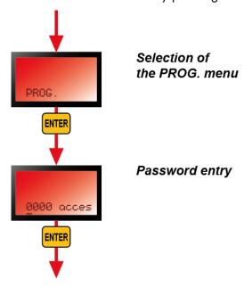
Figure 19: password required (default password: "1000") to access the *PROG* sub-menus. Press *ESC* repeatedly to return to the reading display.
