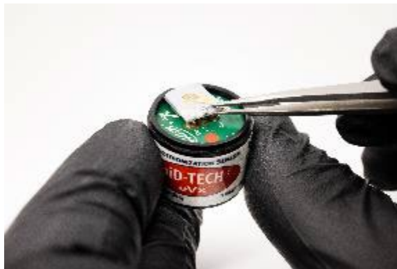
Figure 20 Removal of Cell Assembly
