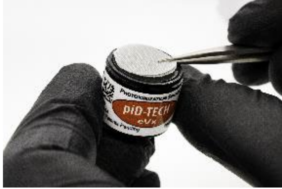
Figure 18 Removal of Filter Media
