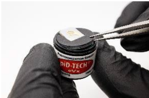
Figure 19 Removal of Spacer
