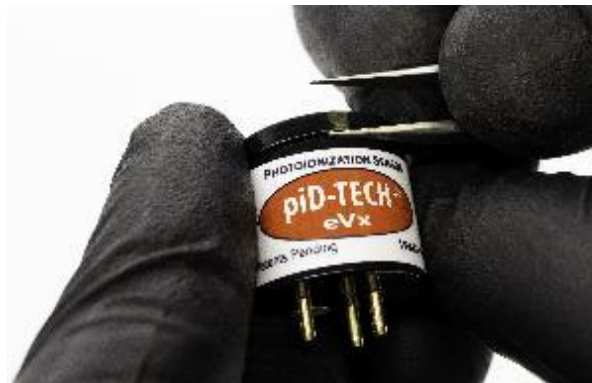
Figure 17 Removal of Filter Cap
