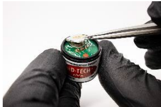
Figure 26 Cell Assembly installation
