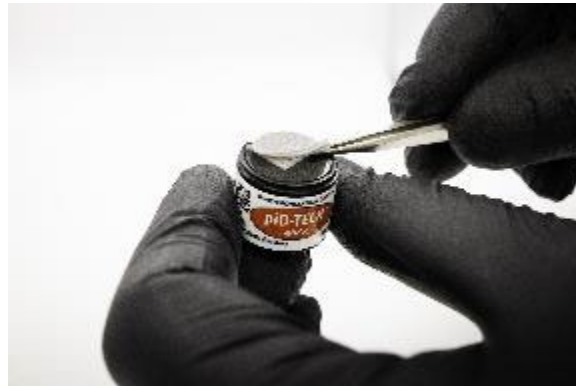
Figure 28 Installing Filter Media
