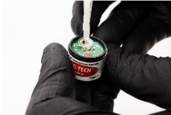
Figure 21 Removal of Lamp
