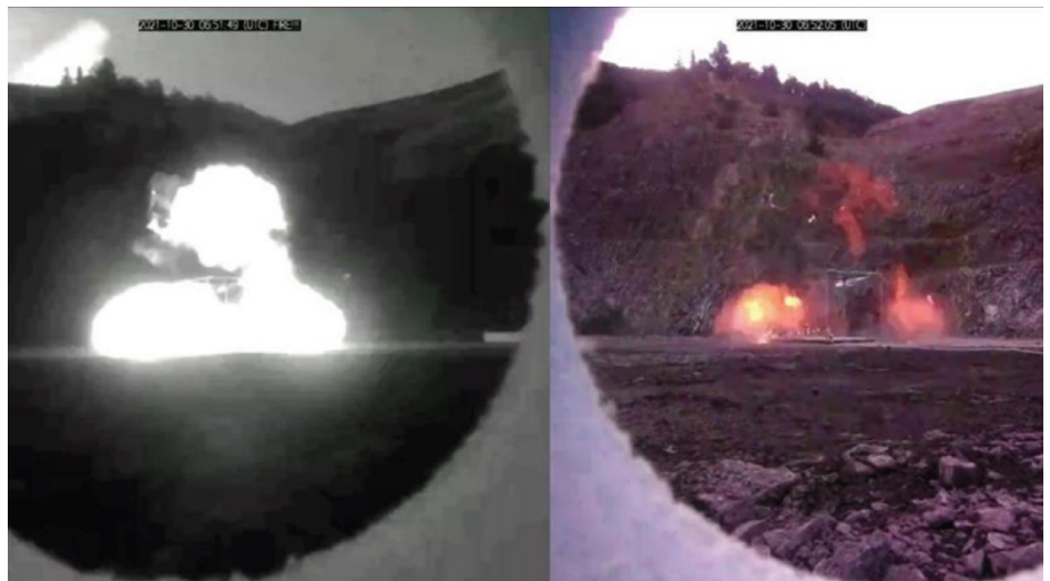
Image of the same hydrogen explosion taken from a near-infrared and a color video
