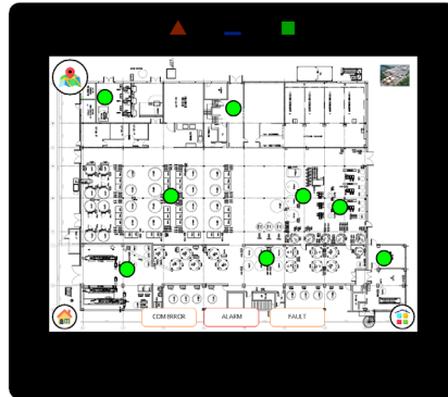
Gas detection layout on-site
