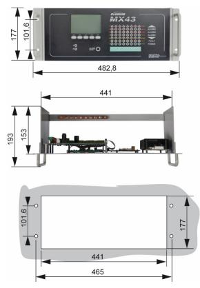
Figure 6: Size of the rack-mounted version.
