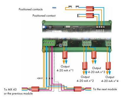
Figure 42: 4-analog output module connections.
