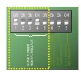
Figure 17: Switches of address configuration.
