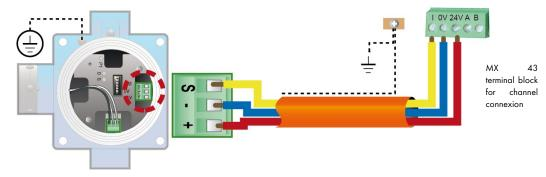
"I" is the 4-20mA signal, 0 and 24V correspond to the power supply.
