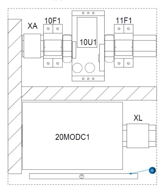
Figure 53 : Implantation of MX43-EB in polyester with AC supply
