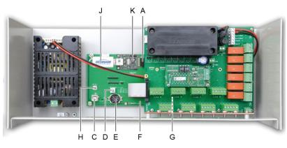
Figure 10: internal view, wall-mounted and rack-mounted versions – microprocessor cards and display.
