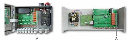
Figure 34: Internal alarm relay connectors (A).
