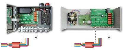
Figure 31: Ground and braid connection.
