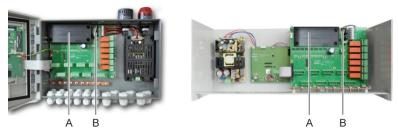
Figure 30: Positioning the battery pack.
