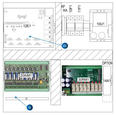
Figure 57: Implantation of the MX43-S in stainless steel
