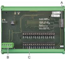
Figure 22: Module of 16 logic inputs.
