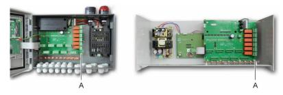
Figure 35: Remote acknowledgement connection (A).
