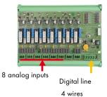
Figure 23: 8-analog inputs.
