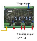
Figure 25: Principle 4-analog output module.
