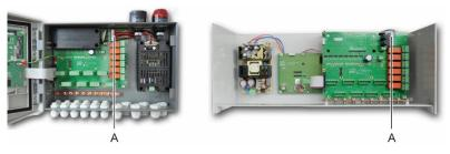
Figure 37: Location of the flash and siren connector (A).
