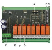
Figure 20: 8-relay module.
