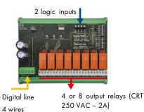
Figure 19: 8-relay module.
